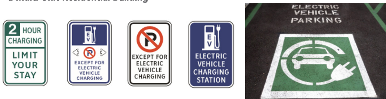
Figure 6: Examples of Mounted and Pavement Signage for Electric Vehicle Charging in a Multi-Unit Residential Building
