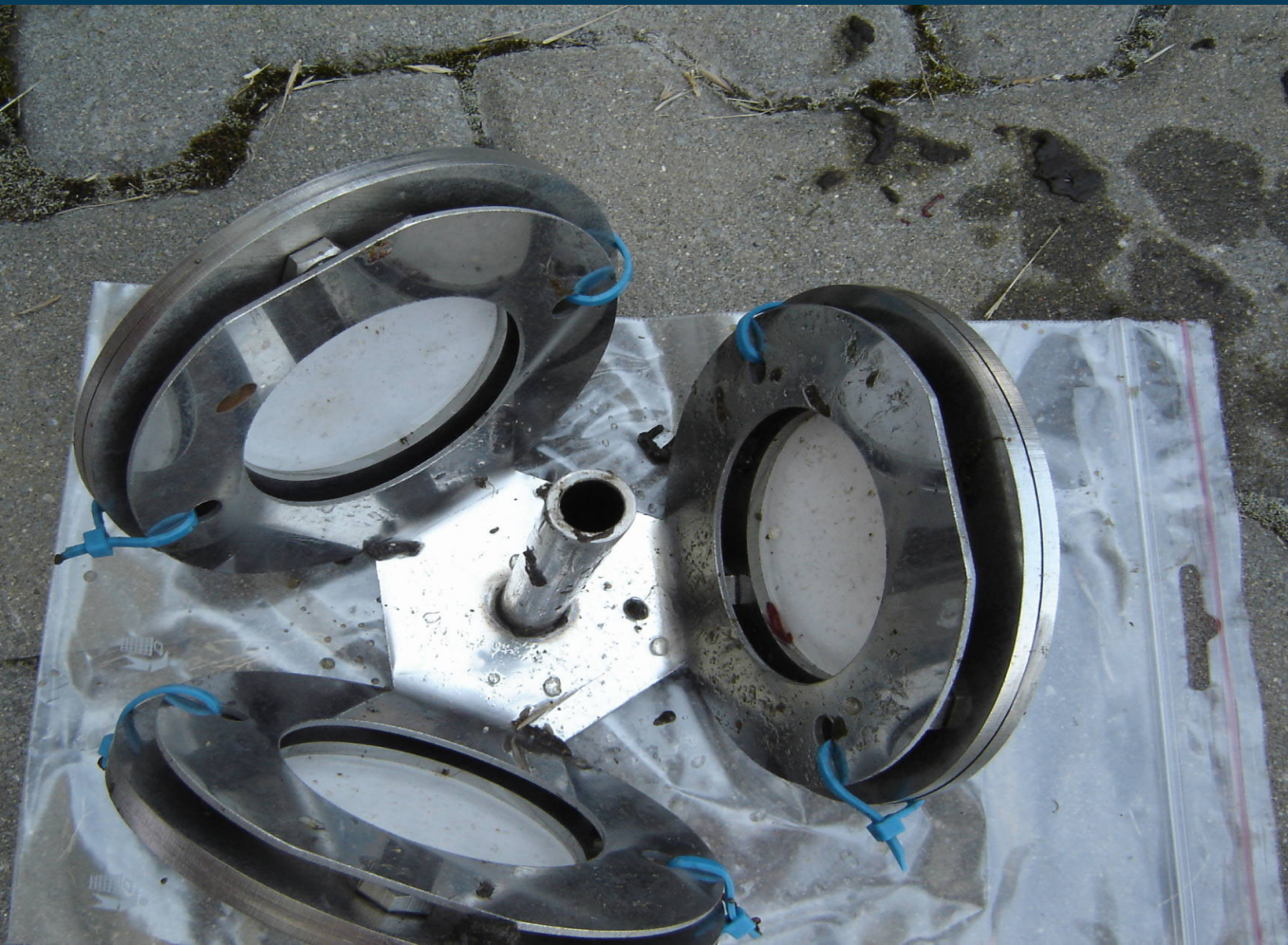
POCIS (Polar Organic Chemical Integrative Sampler) disks mounted in a stainless steel holder for passive sampling
